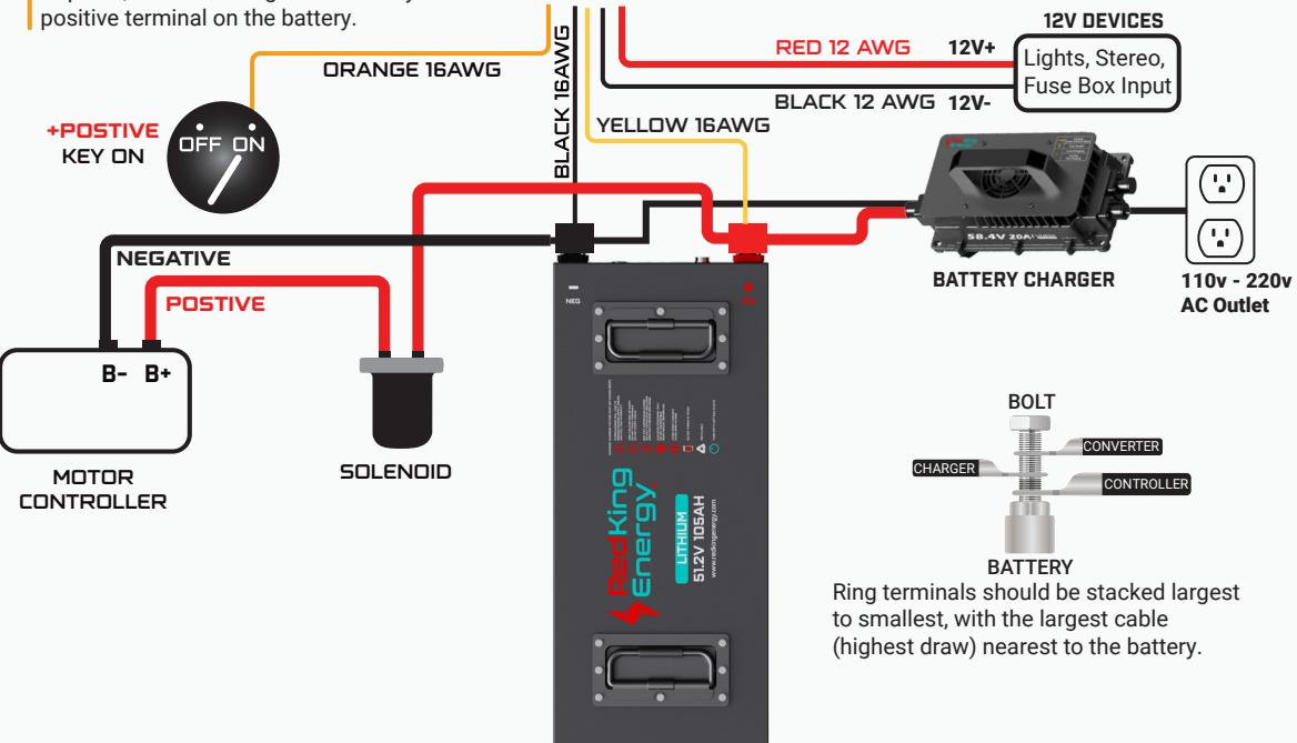
Ring terminals should be stacked largest to smallest, with the largest cable (highest draw) nearest to the battery.
